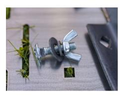
4.) Note the orientation of the carriage bolt, flat washer, lock washer, and wing nut. The lock washer goes against the wing nut. Hand tighten until snug.
