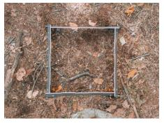
2.) Here is a top-down view of the legs fully interlocked. Be sure that the legs create a square and that the legs are not crooked.
